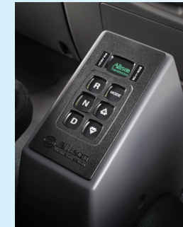
Allison electronic control with digital display
